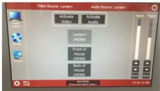
b) Select "Activate Video" and "Activate Audio". Volume of the laptop can be adjusted using the "Program" control on the AVTouchscreen.
