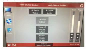
Push "Activate Video" and "Activate Audio" to turn on the projector and lower screen. Select the HDMI location where the laptop is plugged in
